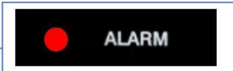
The top LED on the front panel of your Mini Gas Alarm is the ALARM LED. This LED will illuminate red when gas has been detected and the system is alarming.
