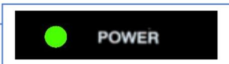
The bottom LED is the power indicator LED, this will illuminate green when the unit is on.
