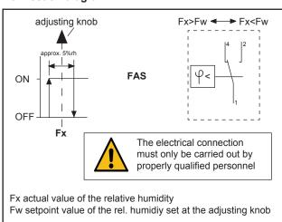
If the rel. humidity Fx (actual value) falls below the setpoint value Fw, contact 1/4 opens and contact 1/2 closes.
